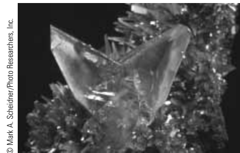
Figure 21.32 The surface that separates the two individual crystals can be considered a type of plane defect. In a perfect crystal, such an interface wouldn't exist.
