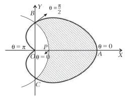
Also both the curves are symmetrical about the initial line (*i.e.*, *x*-axis). The required volume is generated by revolving the upper half of the shaded area about the initial line.
