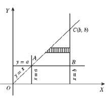
In the integral I we are required to integrate first w.r.t. y and then w.r.t. x. To reverse the order of integration we have to integrate first w.r.t. x and then w.r.t. y. This is done by dividing the area ABC into strips parallel to the x-axis. Let us take strips parallel to the x-axis starting from the line AC (i.e., y = x) and terminating on the line BC (i.e., x = b). Thus for the region ABC, x varies from y to y and y varies from y to y. Hence by changing the order of integration, we have
