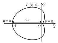
If *s* denotes the arc length of the cardioid measured from the cusp O(i.e.), the point  $\theta = 0$ ) to any point  $P(r, \theta)$  in the direction of  $\theta$  increasing, then *s* increases as  $\theta$  increases. Therefore  $ds / d\theta$  will be positive.
