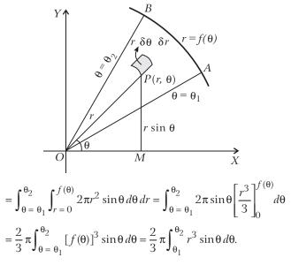
where *r* is to be replaced from the equation of the curve  $r = f(\theta)$ .
