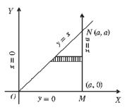
To reverse the order of integration, we have to integrate first w.r.t. x regarding y as constant and then w.r.t. y. This is done by dividing the area ONM into strips parallel to the x-axis. Let us take strips parallel to the x-axis starting from the line ON (i.e., y = x) and terminating on the line MN (i.e., x = a). Thus for this region ONM, x varies from y to a and y varies from 0 to a.
