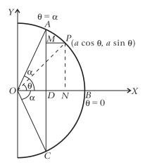
Take any point  $P(a\cos\theta, a\sin\theta)$  on the circular arc ABC which is symmetrical about the x-axis and which subtends an angle  $2\alpha$  at the centre O so that  $\angle AOB = \alpha$ .
