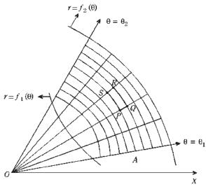
between two consecutive circles and  $\delta\theta$  be the angle between two consecutive lines. There is thus a network of elementary areas (say n in number) of which a typical one is PQRS. If P is the point  $(r,\theta)$ , the area of the element PQRS situated at the point P is  $\frac{1}{2}(r+\delta r)^2\delta\theta - \frac{1}{2}r^2\delta\theta = r\,\delta\theta\,\delta r$ , by neglecting the term  $\frac{1}{2}(\delta r)^2\delta\theta$  being an infinitesimal of higher order.
