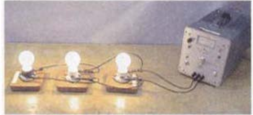
A parallel circuit of light bulbs is shown in above Fig.
